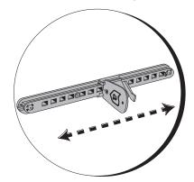
The adjustment lever can be pulled toward you with the opposite foot to create hands-free adjustment, if necessary.
